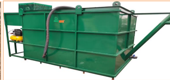
Figure 13 - SNRE, Metal bio gas plant - 60 cumtr capacity
