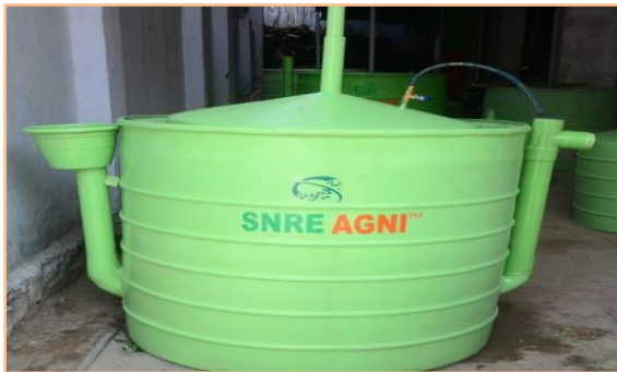
Figure 10 - SNRE, FRP Bio gas plant
