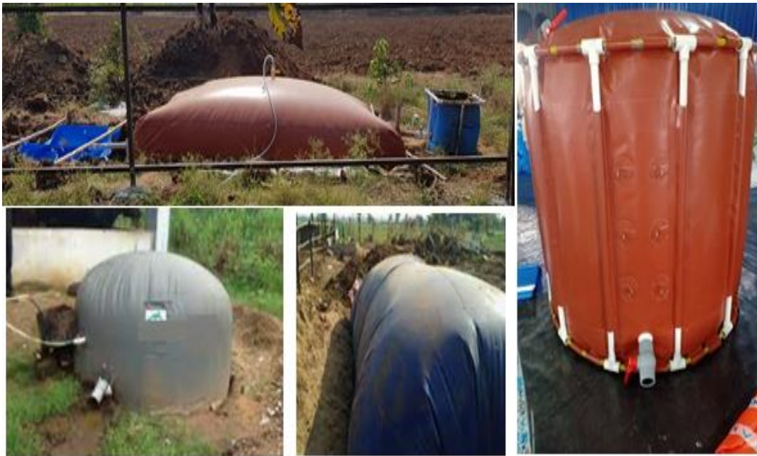
Figure 18 – Different types of balloon Bio Gas Plant- with different methods/ styles of placement & usage
