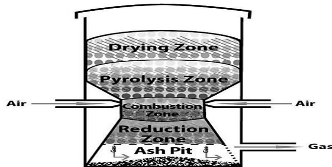
Diagram showing the different zones in the process of gasification in downdraft gasifier.
