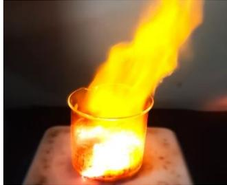
Fig.1 Sample preparation using auto-combustion
